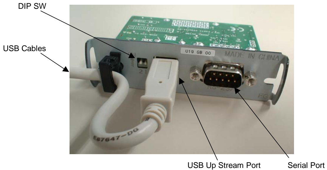
Figure 3.2 External View of USB Interface Board
