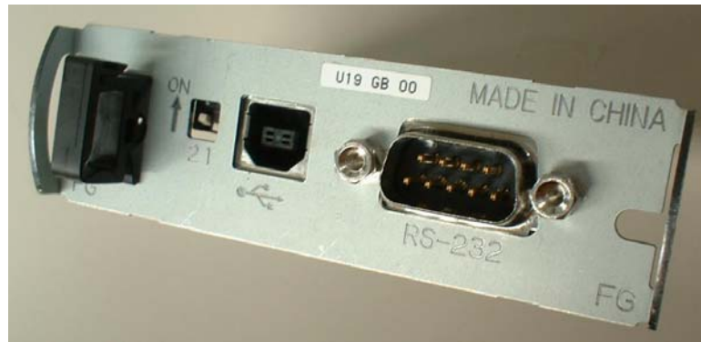
Figure 1.1 UB-U19 Interface Board Structure
